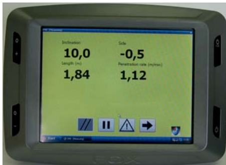
Inklinator CMS Instrument in PC environment Angle and Length measurement with laser/GPS Logging and monitoring function.
