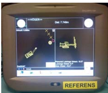
Inklinator CPN Navigation system with: Angle and Length measurement GPS navigation and GPS compass
